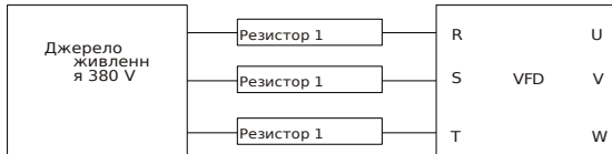
Figure 9-1 380V drive device charging circuit example
