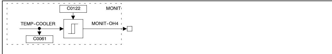
Fig. 2-152 Monitoring of the heatsink temperature, with adjustable threshold (OH4)
