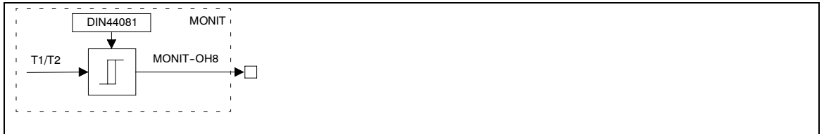
Fig. 2-153 Monitoring of the motor temperature (OH8)
