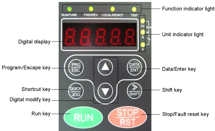
Figure 5.1 Keypad schematic diagrams.
