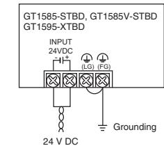
Use the thickest cable possible (max. 2 mm<sup>2</sup>) to minimize the voltage drop and start twisting them close to the connection terminals. Tighten the terminal screws securely with a torque of 0.5 to 0.8 Nm.
